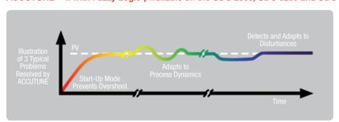
Accutune II provides a new truly plug-and-play tuning algorithm which will, at the touch of a button or through a digital input, accurately identify and tune any process including integrating processes and those with dead-time. This speeds up and simplifies startup, plus allows retuning at any setpoint. Also
